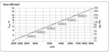
Flow, pressure drop and sound level pressure.
