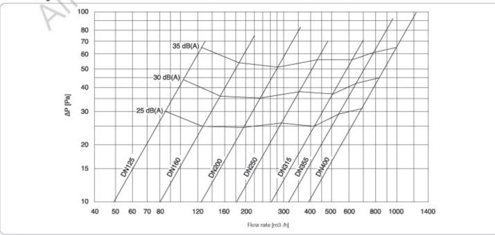
Sound level pressure with 4dB of room attenuation.
