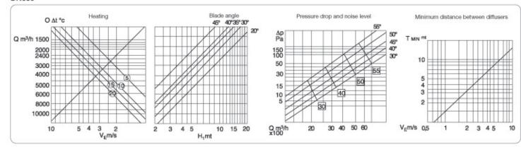
During the cooling phase, consider a blade inclination of between 45° and 55°
